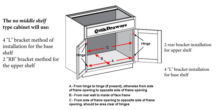
Record the measurement from hinge to opposite side of opening. If there is no hinge, then measure from side of opening to opposite side of opening.
